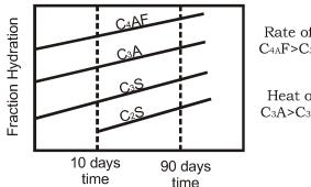
Rate of Hydration C<sub>4A</sub>F>C<sub>3</sub>A>C<sub>3</sub>S>C<sub>2</sub>S
